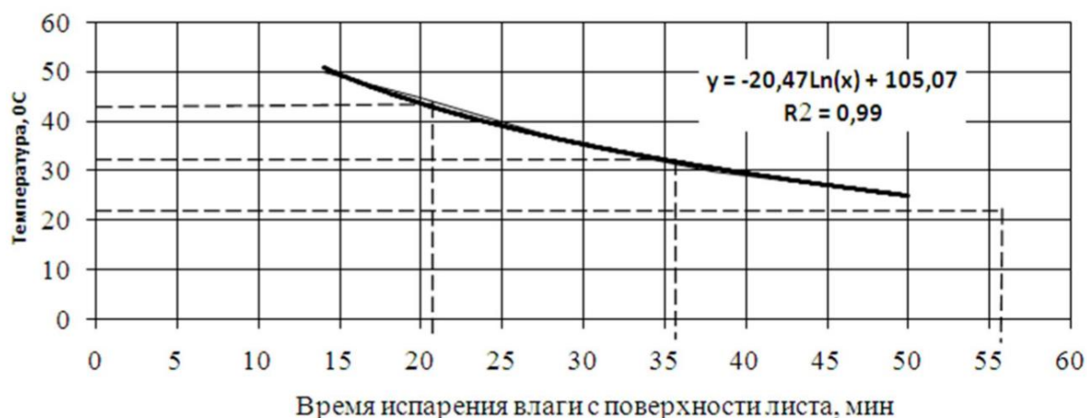
Figure 2 – The schedule of dependence of time of evaporation of moisture from the surface of the square of leaves from air temperature.
