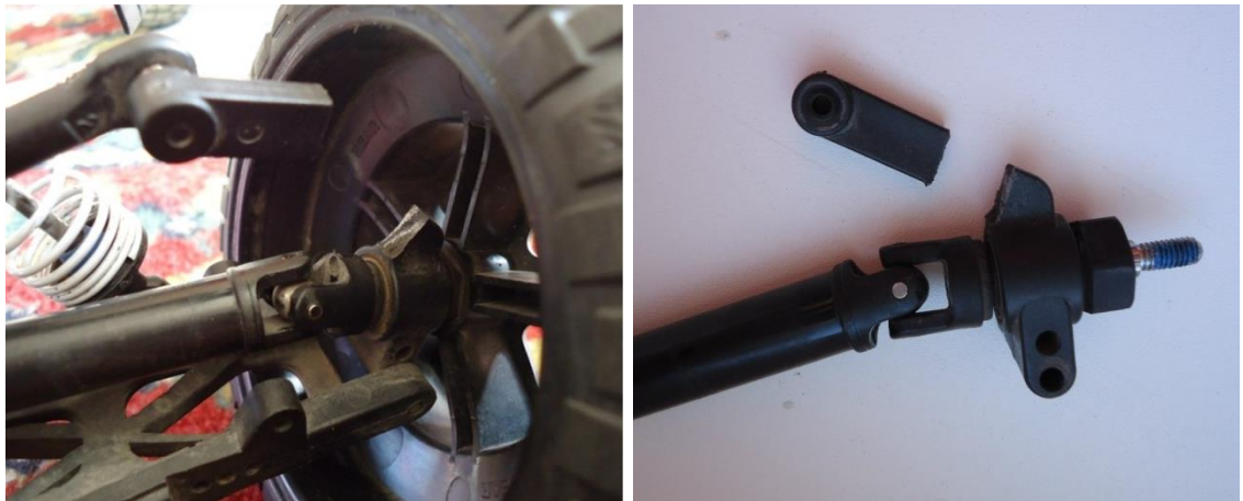
Figure 1 - Suspension unit with the damage of a fragment of the hub of the rear wheel Assembly.
