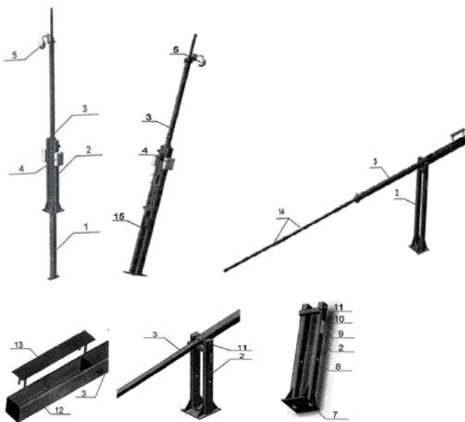
Figure 5 - Support for external lighting and surveillance systems [6]: 1 - base-set; 2 – rack; 3 - the movable part; 4, 5 – electric; 7 – flange; 8 - by-hole; 10 - horizontal limiter; 11 – axle; 12 - opposed to; 13 – cover; 14 – Extension; 15 - Front.
