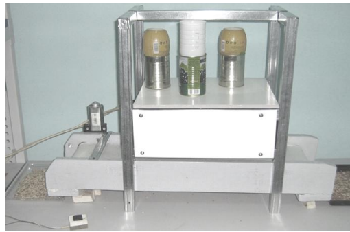
Figure 5 – The elevator model
